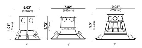
Standard junction box is integrated to downlight for quick and easy retrofit installations
